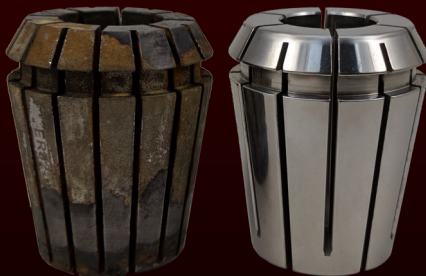
Standard vs Stainless Collets shown were submerged in Chicago tap water for 3 months.
