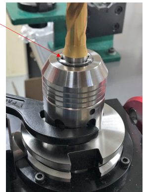
Tighten lock nut until it stops or 1mm (0.040") of the chuck body protrudes out from the face of the lock nut.
