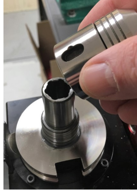
Remove the lock nut from the BC holder assembly, wipe off any dirt or existing grease from taper and inside the lock nut.
