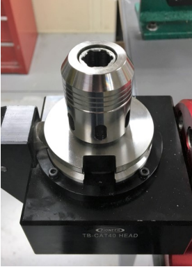
Remove the lock nut from the BC holder assembly, wipe off any dirt or existing grease from taper and inside the lock nut.
