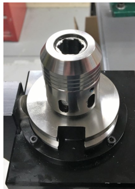
Re-Assemble lock nut.
