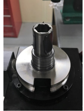
Apply grease to taper.
